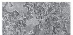
Galvanized G-90 SRI-65 Metallic coating over steel. No finish warranty, no perforation warranty
